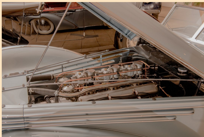
The triple-carbureted V-12 that Mr. Mann believes delivered a French victory in 1938. Credit...Todd Midler for The New York Times
