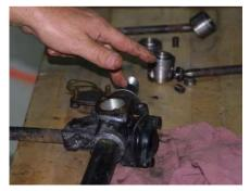
On the later models without lubrication nipples, the two covers just removed can be drilled and tapped for grease fittings. The covers are thick, but be sure that the fitting does not protrude into the working parts. Grease fitting are usually threaded  $\frac{1}{4}$ -28 and the proper tap drill is a #3, but a 7/32 makes the hole easier to tap and works fine.
