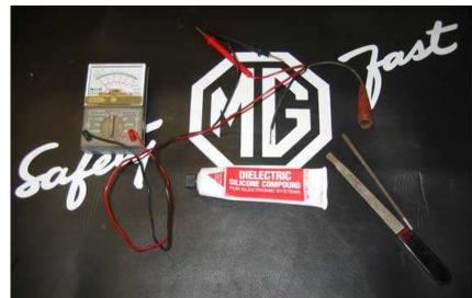
easy to use, and can be priceless when attempting to locate an electrical problem. I found that a short piece of wire with alligator clips on one of both ends also comes in handy for diagnosing bad grounds. Attach one end of the wire to bare metal on the car body (or engine) and the other end to the back of a light housing (the mounting bolts are usually best) or other electrical
