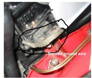
The forked or round connector goes over the bolt on the turn signal housing and is secured by the mounting nut (see octagon in picture) and the bullet connector goes to any black wire behind the grill. Make sure the connector at the housing is making contact with the nut, because some turn signal housings will have a rubber or plastic
