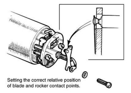
Unscrew the diaphragm by holding it at its base and unscrewing it from the points. Remove the lower portion of the points by pulling the free floating pin out of the pedestal. The top portion of the points is, obviously, held in place by the small screw. Be careful of the two wires coming out of the electro-magnet body. I broke one of the lugs off mine and had to re-solder it. Unfortunately, there is just barely enough wire to reach up to the top of the pedestal.
