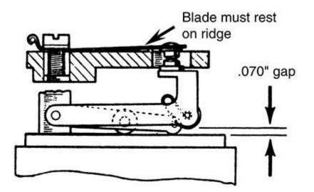
1) Slacken the screw securing the contact blade (upper portion of points or upper contact arm) and swing the blade to one side, so that the points no longer make contact.
